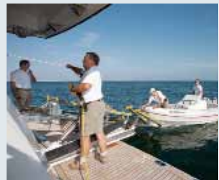
The tender is cradled by a series of rollers and then launched without touching the swim platform.
